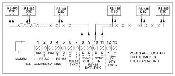
Figure C-9 Using the Master Clock as a Slave to Allow 30 Extra RS-485 Time Synchronizing Devices
